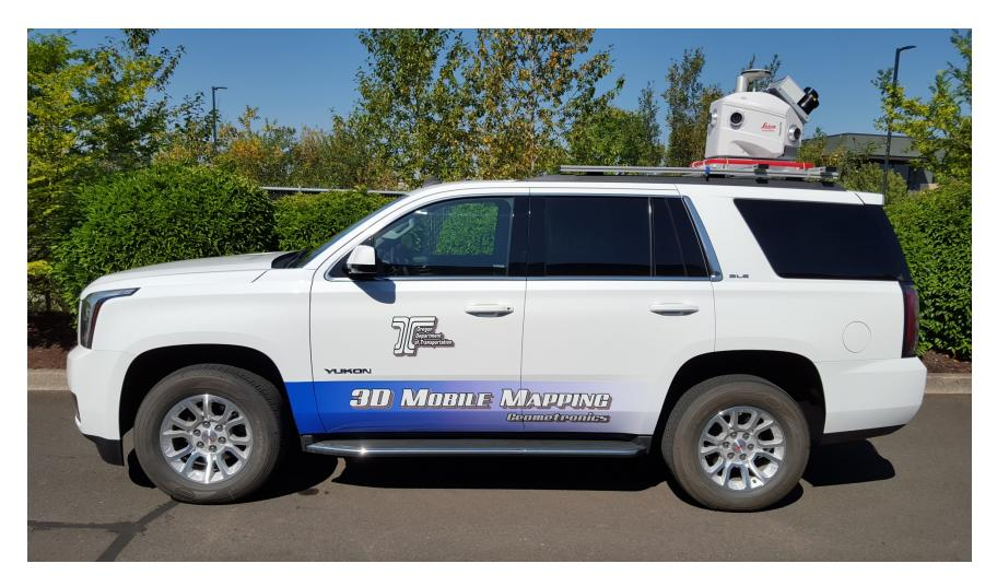
Laser scanner that fires 1.2 million laser pulses per second, 8 cameras that produce a 360 degree image every few feet
